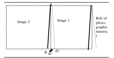
Figure 3: Image Alignment with Rotation
